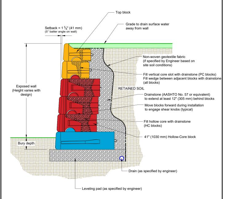
Note: Wall designs typically include a combination of solid, PC, and hollow-core blocks. Redi-Rock blocks are designed to be used together. Block type, size, and configuration will vary based on site-specific conditions and wall height.
