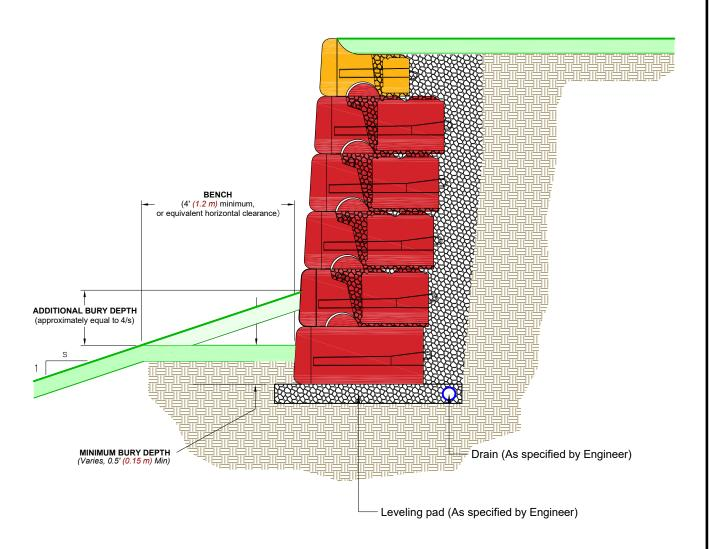
This drawing is for reference only. Determination of the suitability and/or manner of use of any details contained in this document is the sole responsibility of the design engineer of record. Final project designs, including all construction details, shall be prepared by a licensed professional engineer using the actual conditions of the proposed site.
