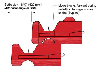
Redi-Rock has two options for large batter retaining walls. Both options are created by relocating the knob so that it is further back in the Redi-Rock blocks compared to our smaller batter walls (5° and less). There are two knob locations further back in the block which create the 9" (230 mm) setback block and the planter block. Blocks made with knobs in either of these locations almost exclusively use 10" (254 mm) diameter knobs.
